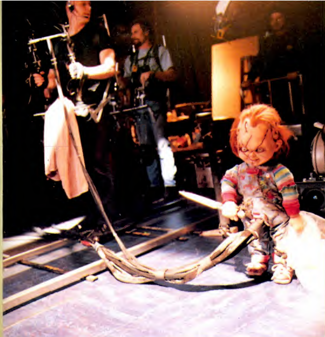
Filming the animatronic Chucky using a cable-controlled walking rig.
